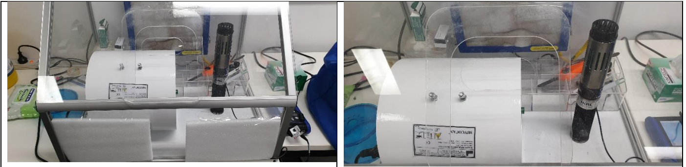
Unit inside sealed enclosure with ozone sensor
